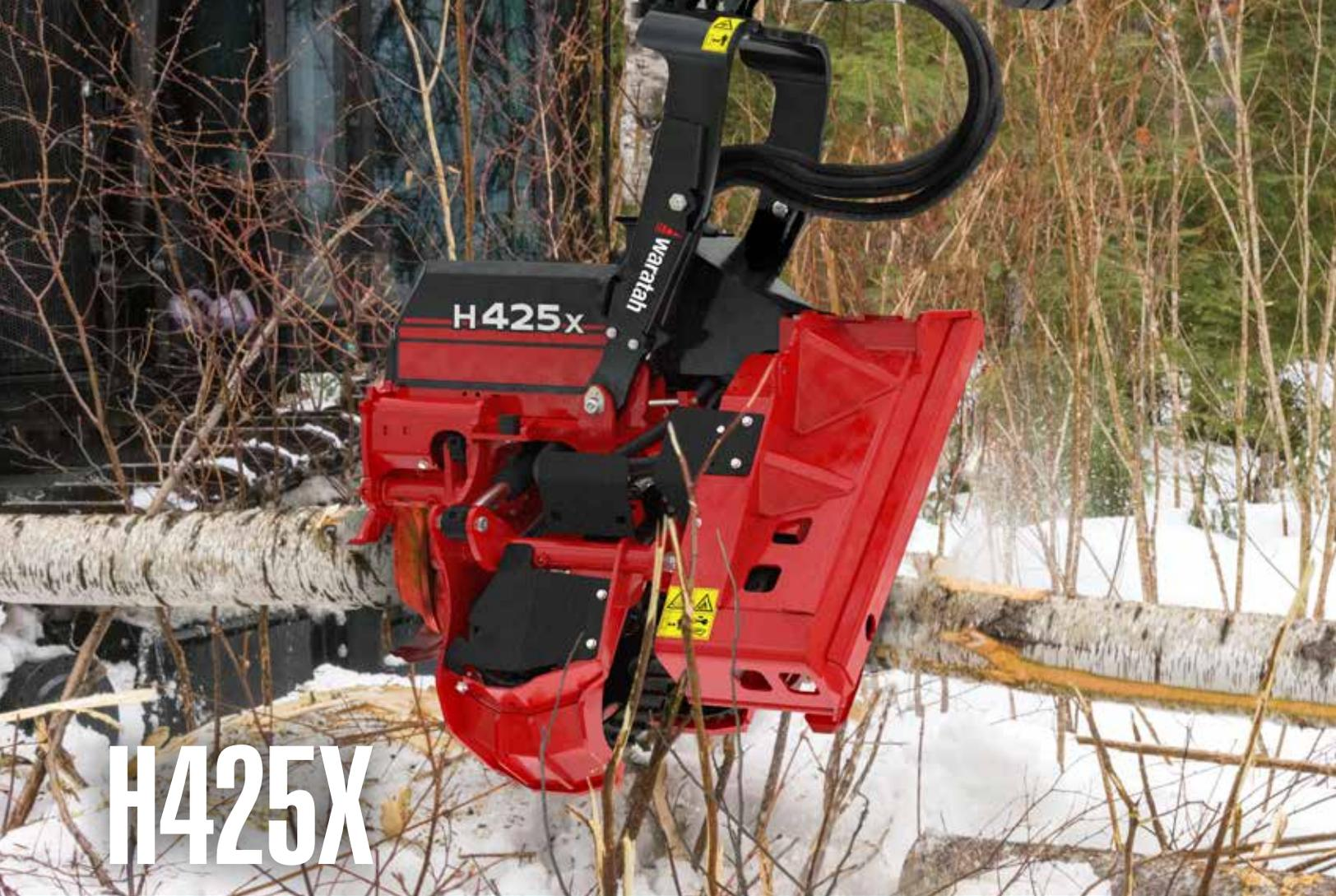
Equally comfortable on track machines, the H425X comes equipped with an extreme duty main saw box and excels in mixed stand harvesting. With a powerful control valve, high-performance drive motors, precision delimiting and optional top saw, “backing up” will not be in your vocabulary.
