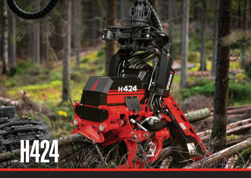
Characterized by its consistent performance and skill set in second thinnings and early regeneration cuttings, the versatile H424 is equally suited for processing or debarking applications. With a durable frame, well-protected hosing, feed power and ample cutting capacity, it's a very capable all-around head for mid-sized harvesters.
