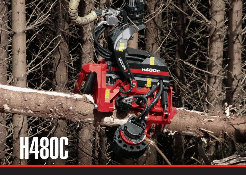
Experience counts, and the popular H480C is no exception. This aggressive head well-known for its large diameter capacity, optimized feed force and processing speed gives excellent and unprecedented tree processing especially in crooked timber.
