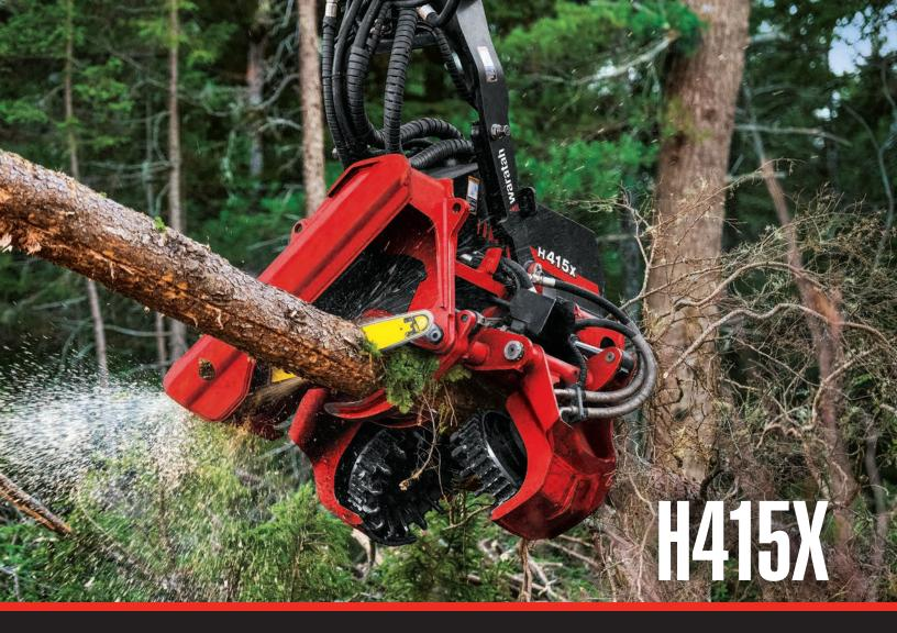
Equally comfortable on track machines, the H415X comes equipped with an extreme duty main saw box and excels in mixed stand harvesting. With a powerful control valve, high-performance drive motors, precision delimbing and optional top saw, "backing up" will not be in your vocabulary.
