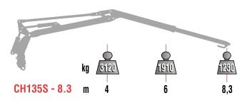
Actual lifting capacity depends on which link, rotator and harvester head is used.
