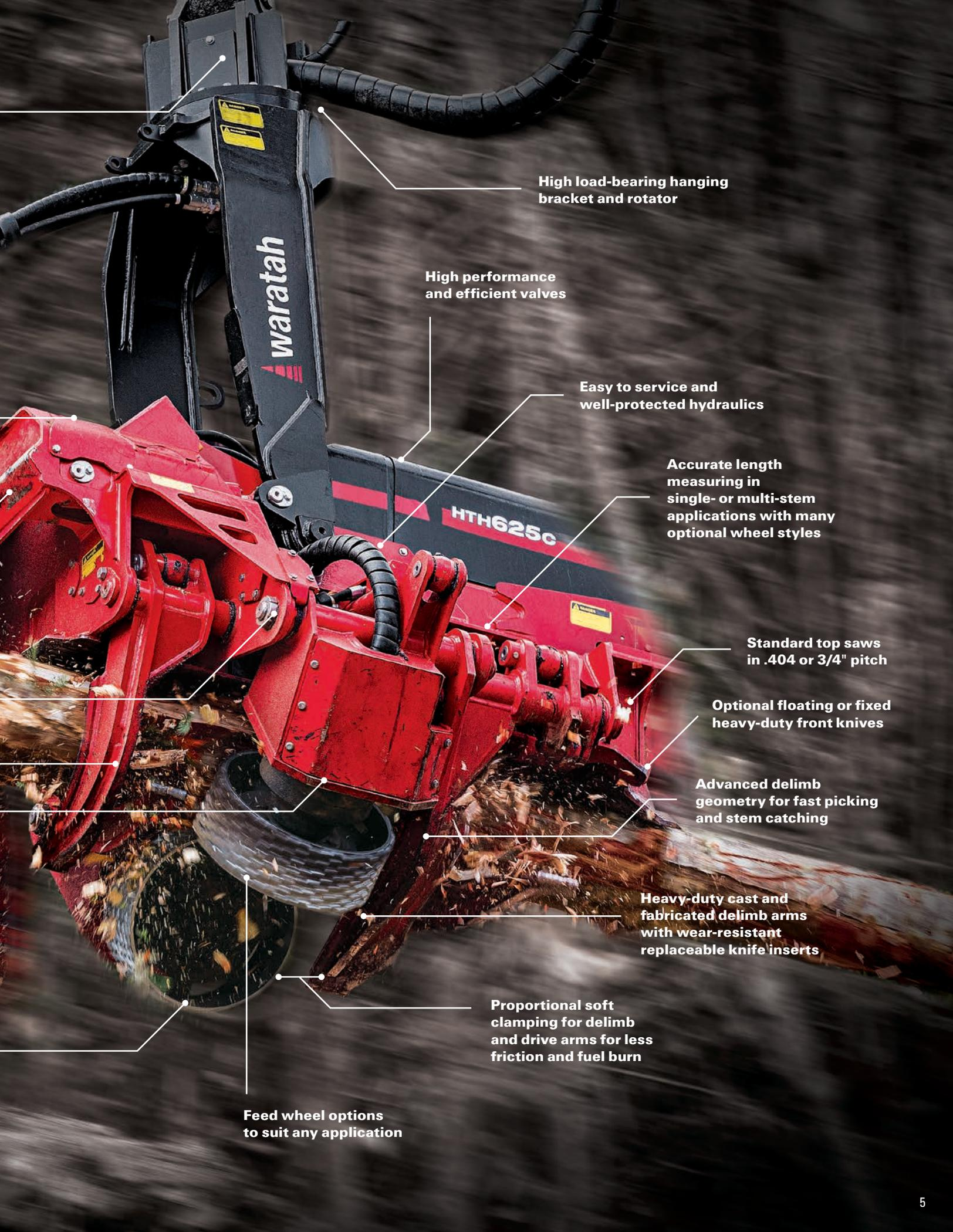
High load-bearing hanging bracket and rotator
