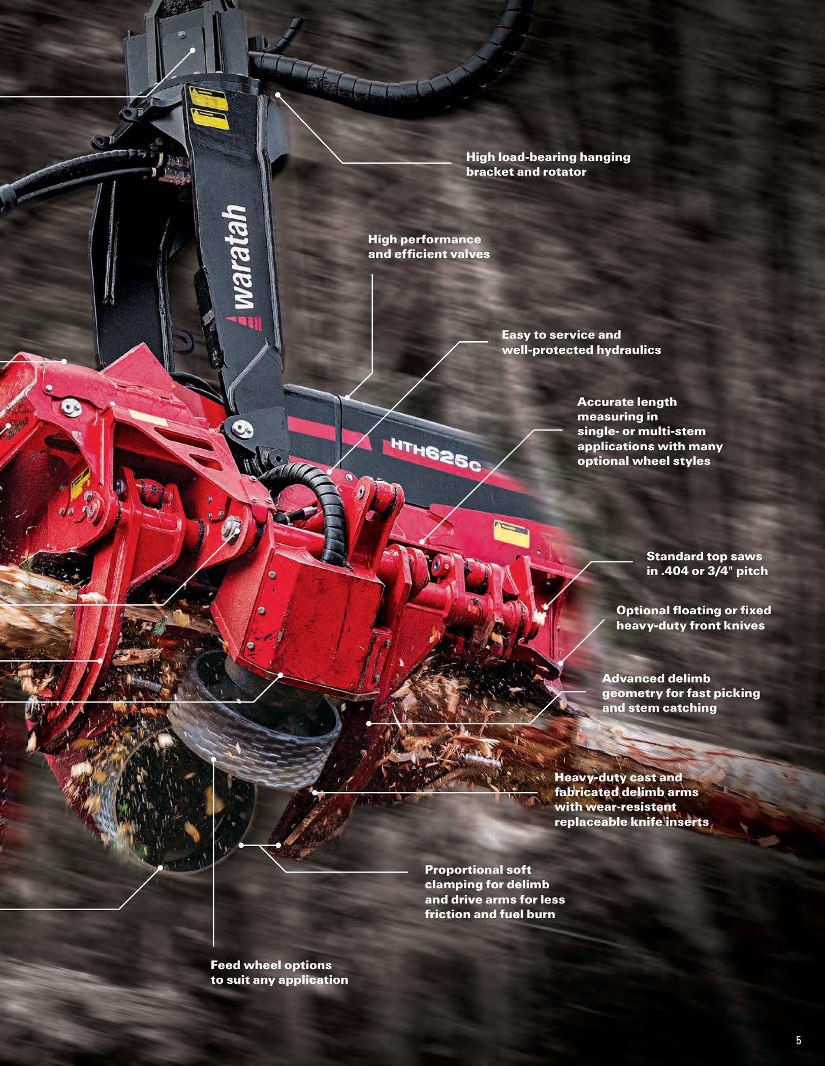
High load-bearing hanging bracket and rotator
